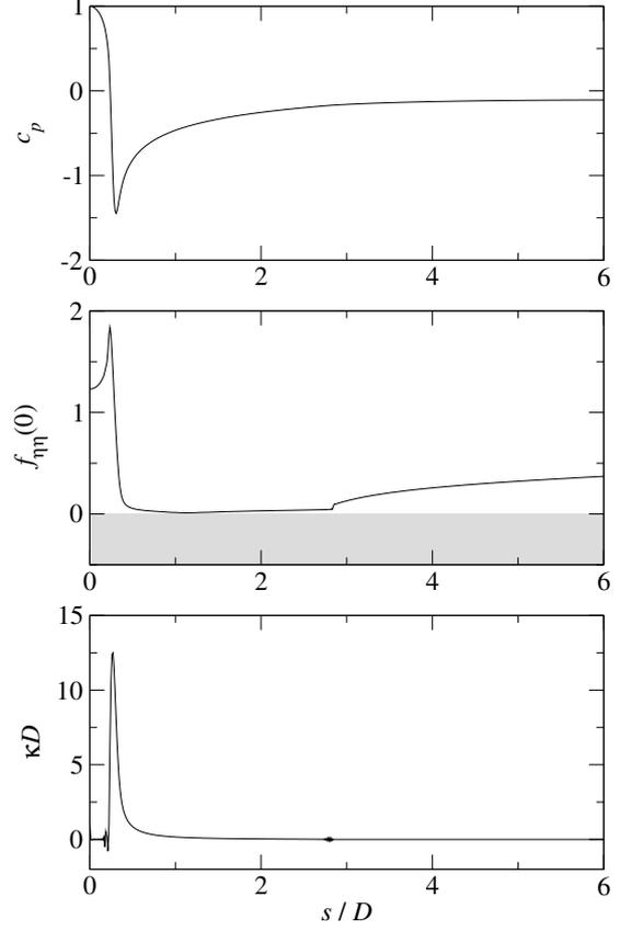
Figure 5: Pressure coefficient, shear stress, and curvature after 30 iterations in the plane-symmetric case. The junction is located at  $s_0/D = 2.84$ . The shaded area indicates separated (infeasible) solutions.
