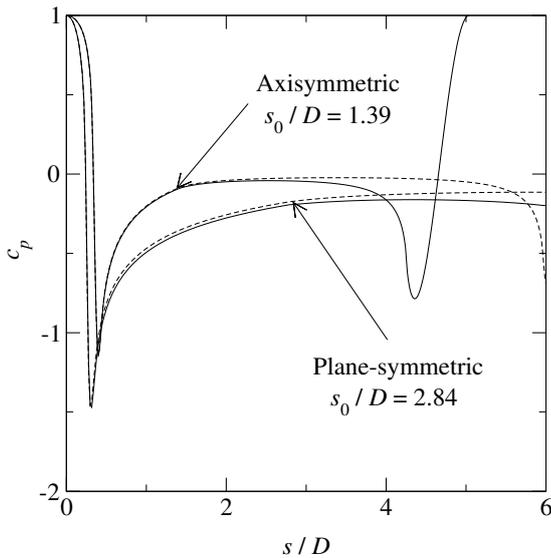
Figure 7: Effect of aftbody length on pressure coefficient profiles for plane-symmetric (solid line,  $L_A/D = 5.39$ ; dashed line  $L_A/D = 8.56$ ) and axisymmetric (solid line,  $L_A/D = 3.38$ ; dashed line  $L_A/D = 5.09$ ) cases.
