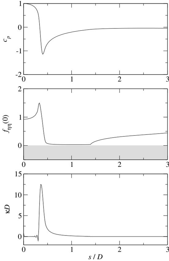
Figure 6: Pressure coefficient, shear stress, and curvature after 30 iterations in the axisymmetric case. The junction is located at  $s_0/D = 1.39$ . The shaded area indicates separated (infeasible) solutions.
