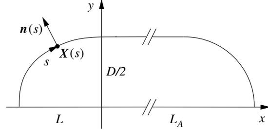
Figure 1: Geometry definition. The  $x$ -axis is the plane or axis of symmetry.
