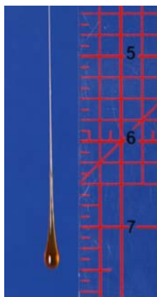
FIG. 5.3. Dripping golden syrup from a knife. The drop shape is paraboloidal, in contrast to the globular shape of glycerine dripping from a capillary tube as in [12]. Note that the scale is in inches.
